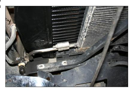
Bolt the radiator to the CAC. Use the 2 new M8 x 35mm bolts (1100035) and M8 washers (1462609) supplied and bolt the CAC to the upper tie bar.
