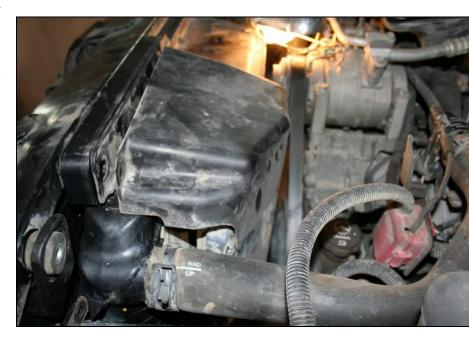
With a 10mm socket, install the hood latch with the 3 bolts taken off earlier (The position is critical, make sure it lines up to the tie bar paint pen marks).
