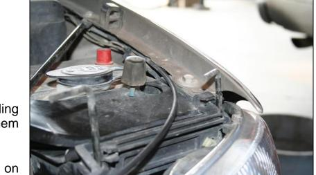
Remove the headlights by pulling the mounting pins to detach them from the mounting panel.
