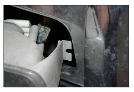
Install the marker lights by tucking in the inside tab first, and then push the outer clip into the headlight panel.
