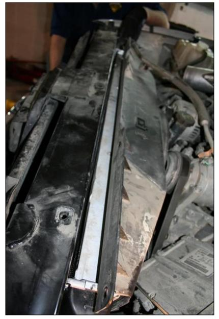
Remove the 2 brackets that secure the bottom of the radiator to the CAC. Unbolt the radiator from the CAC, followed by the 2 bolts that secure the CAC to the upper tie bar with a 13mm socket.
