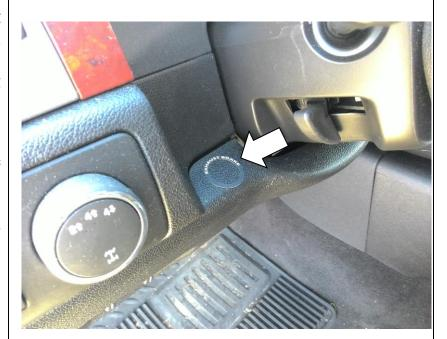
8. Plug the white connector from the VVB harness into the back of the switch and secure wiring with supplied zip ties under the dash.
