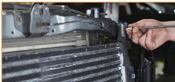
5. Lift the intercooler and remove it from the vehicle. See that both pipes are off the end tanks. You may need to jiggle the intercooler as you remove it to get the pipes off.
