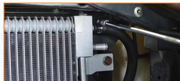
13. Install the other provided hose to the second transmission cooler line. (1x worm gear clamp)
