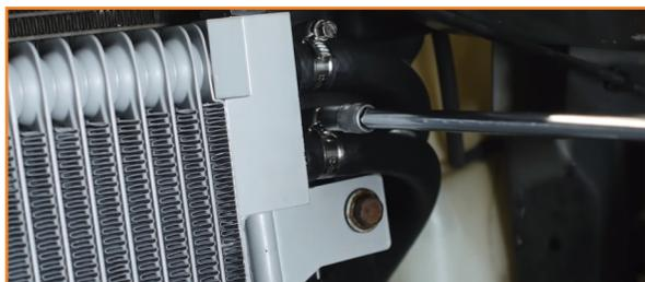
15. Reinstall the cold-side pipe. (1x t-bolt clamp)
