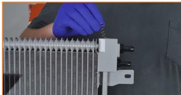
24. Lower your bypass plug into the recess opening.
