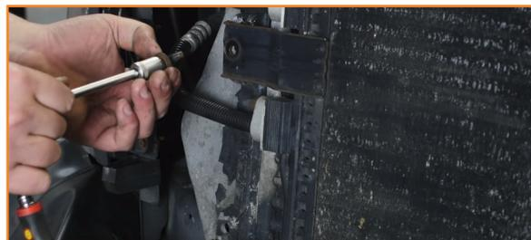
2. Lift the AC condenser up and out from behind the front bumper. Then softly lower it and let it rest so that it is out of the way of the intercooler.
