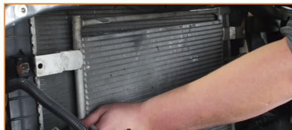
9. Install the stainless-steel hose barbs provided in your kit to the transmission cooler hoses. (2x worm gear clamps)
