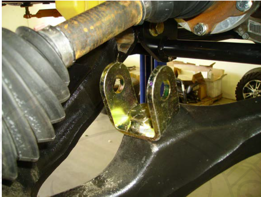
Figure 1: Clevis in lower a-arm, don't tighten yet.
