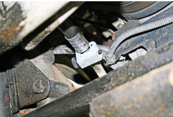
Unbolt transmission line bracket from motor
