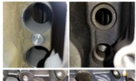
LML (LEFT) STRAIGHT LIFTER BORE, L5P (RIGHT) STEPPED LIFTER BORE.
