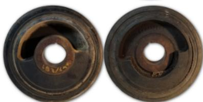
LBZ/LMM - 180DEG COUNTERWEIGHT, 65MM THICK
