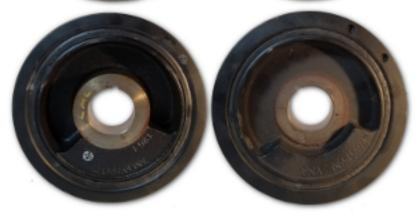
LML - 120DEG COUNTERWEIGHT, 60MM THICK
