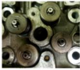
LLY - LML INJECTOR BORE - THREADED BOSS TOWARD INTAKE PORTS BEST PRACTICE FOR POSITIVE ID IS TO REFER TO CASTING NUMBER.
