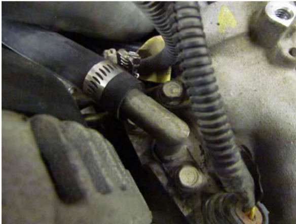
Step 19: Attach coolant return line to modified coolant pipe as shown. This coolant line will route directly to firewall.
