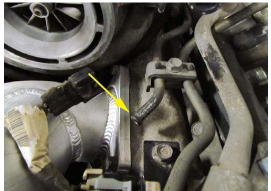
Step 10: Cut end should be similar to above. While not necessary, it is recommend to use flair tool to form end as shown.
