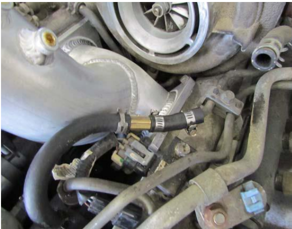
Step 18a: Connect T-Fitting to fuel return lines. Detailed routing is shown on right.
