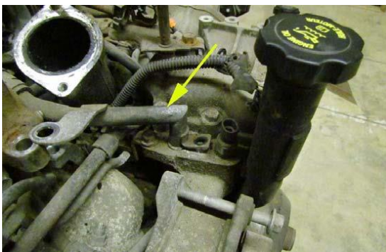
Step 11: Remove thermostat coolant pipe as shown. Pry out with pry bar.
