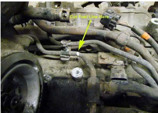
Step 9: Cut fuel line as shown using hack saw or similar device.
