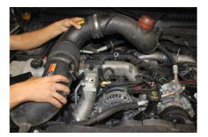
**Step 2:** Remove the intake tube and silencer as shown in photo above.
