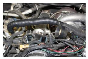
**Step 6:** Wrap large wire loom (D) over wires and wrap loom with electrical tape.
