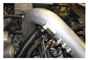
**Step 13:** Install MAP sensor in mounting flange as shown. Hook up alternator power cable. Reinstall intake assembly. Install plugs (H) using Teflon tape as required. On newer LMM's, insert Grommet (G) into hole in mounting flange and install MAP sensor tube into Grommet.
