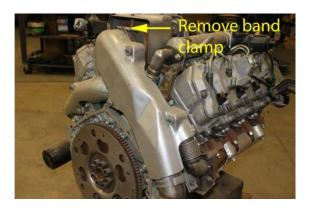
**Step 2:** Remove down pipe assembly and heat shield by loosening band clamp on top. Heat shield does not have to be removed from pipe.
