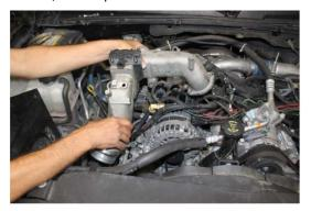
**Step 3:** Loosen clamp on inter-cooler connection at bottom of intake tube. Remove bolts/nuts holding intake tube and remove complete assembly.
