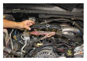
**Step 5:** Open plastic wire harness shield and remove from vehicle.
