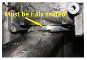
**Step 9:** Now loosely install new tube assembly. Make sure intake tube with O-rings is fully seated into 'Y' bridge. Picture above shows unacceptable gap. Pry bar may be needed to insure proper fit.
