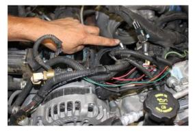
Step 4: Remove stud from mounting flange as shown.
