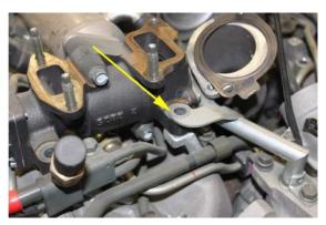
**Step 4:** Remove bolt holding bracket as shown. Remove heater hose from cooler and lift assembly off.
