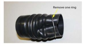
**Step 10:** To facilitate installing the tube assembly unto the Lower boot, remove one of the metal rings as shown above. This will allow the tube to slide further into the boot creating more attachment surface for the clamp.
