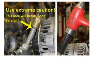
**Step 3A:** Remove brass fuel test port carefully. Install deep socket on fitting and hit with hammer to break the fitting loose. Unscrew fitting carefully so as not to break at stem. Install fuel test port cap (F) in same location snuggly.
