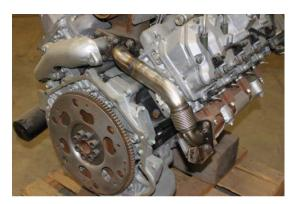
**Step 5:** Mount new LB7 up pipe to exhaust manifold and turbo pedestal with 28 ft-lbs.
