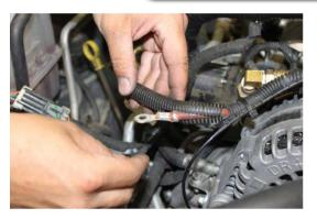
**Step 7:** Install small wire loom (E) over grid heater power cable. Make sure spade lug is completely covered. Wrap tightly with electrical tape.
