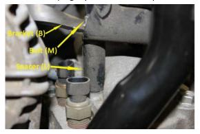
**Step 8A:** LBZ only - Install spacer (L) using Bolt (M) as shown on LBZ only. Use existing spacer on all other models.
