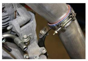
**Step 12:** Install band clamp and isolator (A) to bracket as shown. Tighten band clamp to tube.
