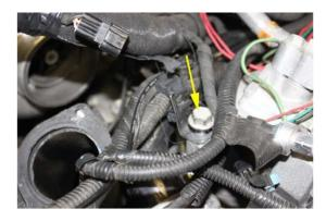
**Step 8:** Remove back bolt on A/C compressor which holds wire harness bracket as shown.
