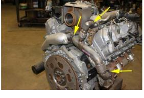
**Step 3:** Remove bolts from flanges at exhaust manifold, turbo pedestal and EGR cooling tube. Remove assembly.
