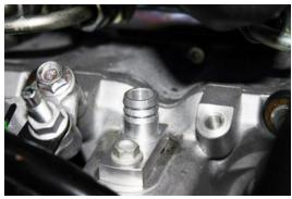
Step 3: Mount the billet fittings using the 6mm bolts removed in step 2 as shown. One for each valve cover.
