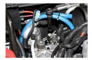
Step 7: Attach the shorter hose to the fitting on the passenger side and attach with supplied hose clamp. Join the two hoses together with zip ties and run parallel as shown above.
