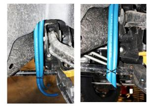
Step 4: Install the cap supplied with kit using a zip tie as shown by arrow. Snug the zip tie with pliers and cut off excess.
