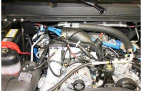
Step 6: Attach the longer hose to the billet fitting on the driver side and attach with supplied hose clamp. Route the hose behind the air tube as show in above photo.
