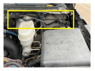
5. Route the single black wire exiting the relay down along the frame rail to the rear of the vehicle. Secure the wire along the way with provided zip ties.
