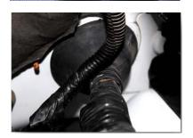
Route the Dirty Alli-Locker wire harness behind the dash panel and through the firewall. We recommend going through the grommet on the drivers side shown in figure 2.
