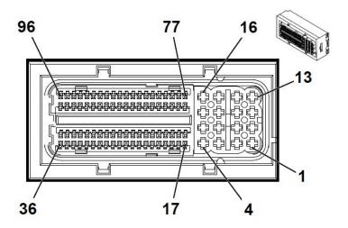
For use only with SoCal Diesel® Alternative Firing Order Camshafts **96 Pin Black Connector K20 Engine Control Module X2**. Number designations can also be found on the back of the connector.
