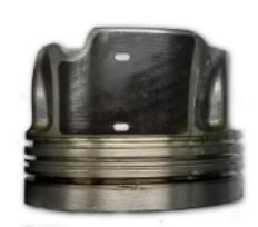
LML - NARROWER, COATED SKIRTING, EARLY NOTCHED ON 1 SIDE FOR PISTON SQUIRTER, LATE NOTCHED ON BOTH SIDES
