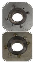
THE FUNCTION OF THE RELUCTOR WHEEL IS TO SWEEP A SENSOR THAT TELLS THE PCM WHERE THE CRANK IS IN ITS ROTATION. IN HIGH RPM/HIGH POWER APPLICATIONS, WE USED TO WELD THE BOLTS IN. AS YOU CAN SEE, THE WELDS FAILED AND BROKE 2 BOLTS. THIS WAS IN CHEAP HOOKER AND THE BEHAVIOR WHEN IT FAILED SEEMED LIKE A BROKEN CRANK. AS A RESULT OF THIS EXPERIENCE, WE NOW INSTALL THEM WITH 6 BOLTS WITH THREAD LOCKER AND HAVE NOT EXPERIENCED A FURTHER FAILURE.
