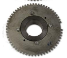
LML - FOUR BOLTS, HUB DOES PROTRUDE INTO WHEEL
