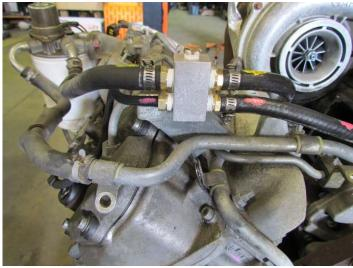
Install new hoses from kit as shown using supplied clamps.
