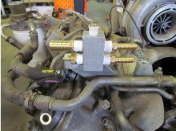
Install fittings using Teflon tape as shown.
