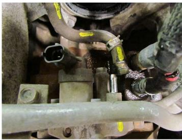
Remove supply line to CP3 off pump.
