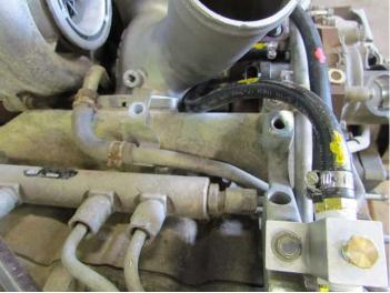
Reassemble Y-bridge, mouthpiece, and check for leaks.
