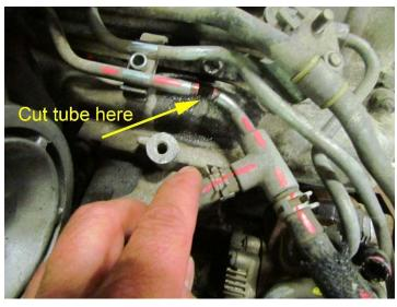
Using compact tubing cutter such as  $\underline{\text{DHD 35030}}$  , cut the supply tube as shown.
