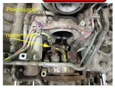
Image above shows DHD 700-125 Standard Fuel Block Upgrade kit. DHD 700-155 Super High Flow kit is similar
