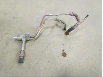
Stock assembly can now be removed from engine.
