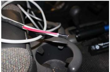
Use electrical tape to bundle the ends of all 6 wires in the harness as shown. Attach connectors back unto switches and insert wire harness through hole. Snap switch panel back in place.
