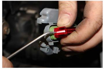
Remove pin alignment piece by depressing retaining tab using a pick as shown. Top connector has red retainer (shown above) and bottom connector is clear. Pin numbers are molded into connector. Locate pin no. 32 on top connector. Lift plastic pin retainer with pick and push pin through back of connector.
