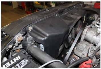
Remove Transmission Control Module cover by removing two bolts on top. Remove both connectors on TCM.
