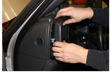
Disconnect battery. Tilt steering wheel fully down, turn ignition key on and put shifter in 1st gear. Remove trim plate by pulling back as shown.
