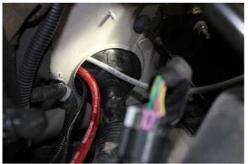
Route wire harness under steering column and through large grommet in the firewall. Grommet is located outboard of steering column and near the top of the firewall. See photo on left.
