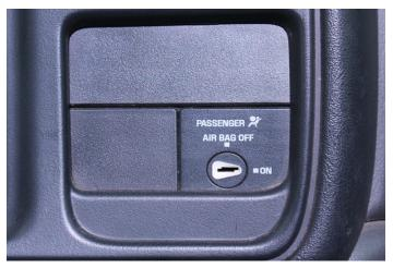
Remove the panel shown above by pulling towards you. It is held in place by retainer clips only. The panel has several configurations depending on options. Unplug connectors in rear.
