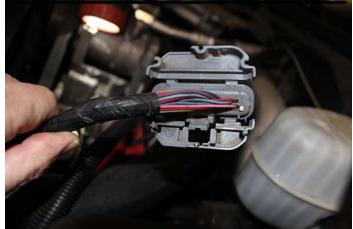
Open rear cover on connectors to expose wires as shown.
