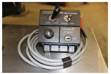
Unsnap any switches attached to old panel. Remove the blank covers from new panel and snap in switches as shown. Leave the blank covers in place if needed.
