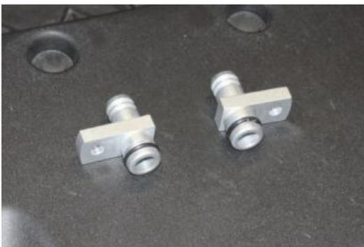
Here are the two billet fittings that will be used to mount the new hose. The O ring ends will be mounted into the valve covers. It's a good idea to put a little oil on the O rings to facilitate installation.
