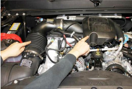
Step 1: Remove the intake tube and silencer as shown in photo above.
