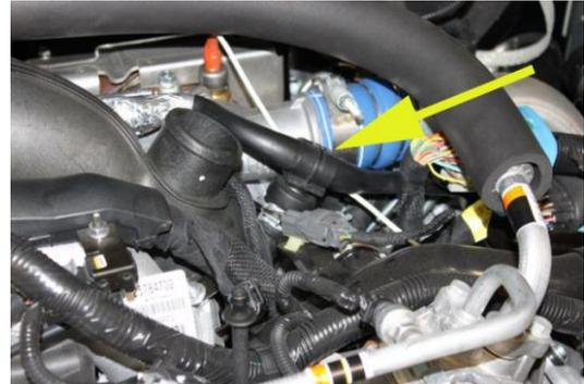
Step 2: Remove the PCV crossover tube by removing 6mm bolts on each valve cover and loosening hose clamp in center (see arrow). The 6mm bolts will be needed later.
