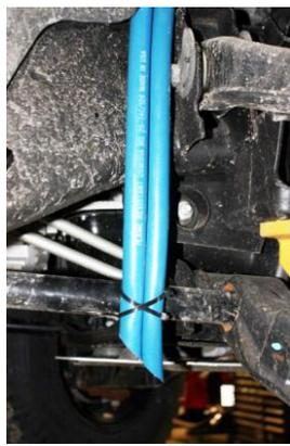
Step 8: Route the hose through the wheel well on outboard side of frame and at rear of upper control arm as shown on left photo. Make sure to route on outboard side of frame to properly clear the exhaust system.
