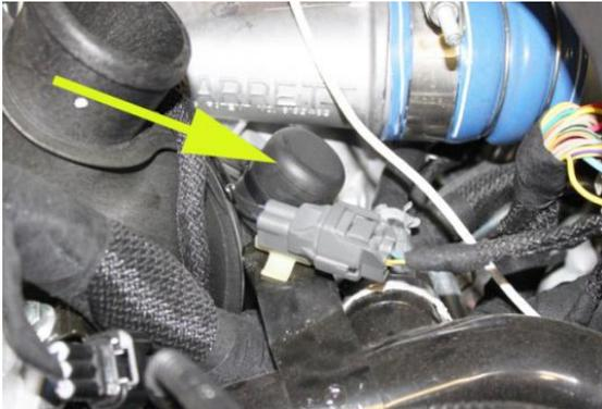
Step 4: Install the cap supplied with kit using a zip tie as shown by arrow. Snug the zip tie with pliers and cut off excess.
