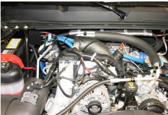
Step 6: Attach the longer hose to the billet fitting on the driver side and attach with supplied hose clamp. Route the hose behind the air tube as show in above photo.
