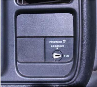
Remove Dash surround bezel by pulling rearward to release clips. If air bag switch is installed as shown in figure 1, remove it. Remove one of the cover plates on Dirty Alli-Locker and snap the air bag switch in the opening. Snap the Alli-Locker in the opening and replace dash surround bezel.
