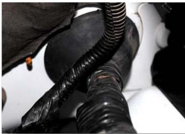
Route the Dirty Alli-Locker wire harness behind the dash panel and through the firewall. We recommend going through the grommet on the drivers side shown in figure 2.
